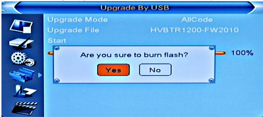
13. Upgrade process starts writing data to the HVBTR-1200. Note progress bar and warning **Do not power off:**
