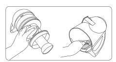
When the cyclone sepatator has been cleaned and dried completley, re-attached the dirt container to the lid of the separator and return the dirt container to the unit.
